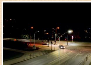
During the modernization of lighting in 137 streets in the town of Alytus, 1,515 units of sodium lamps were replaced by LED lamps and 73,465 m of new electrical cables were laid. Energy consumption was reduced by 46.79%. This represents annual savings of around 45,000 € per year.
